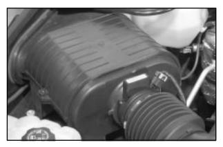
The engine air cleaner/filter assembly is located in the engine compartment on the passenger's side of the vehicle. See "Engine Compartment Overview" in the Index for more information on location.
